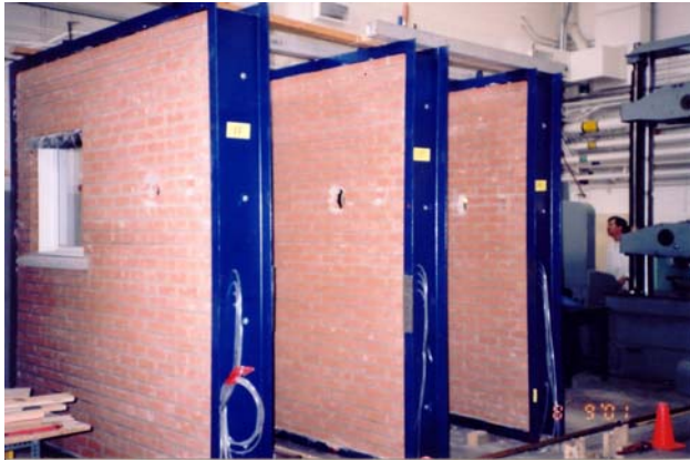
A series of wall assemblies with brick masonry veneer were constructed and tested for the MEWS project. Flaws were deliberately introduced to assess the moisture management performance of the various wall assemblies.
