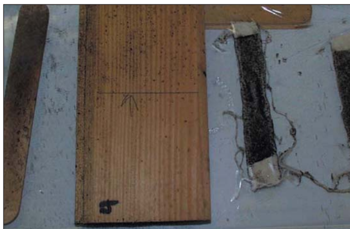
All samples of wood, gypsum and moisture-resistant drywall showed fungal infection, whereas all masonry samples showed no traces of mould. This wood tongue and groove sample (Sample 3) showed “severe growth” of fungal infection on the cut ends.
