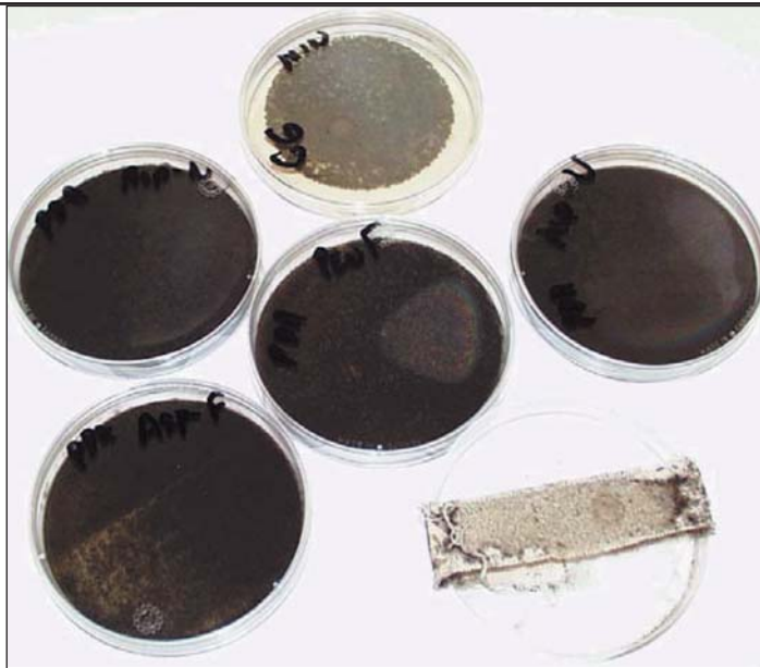
Testing in the FMRT study was completed on seven commonly used building materials, with a 28 day incubation for each sample.
