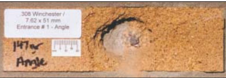
Above photo shows entrance point of impact. Bullet failed to pass through brick wall.
