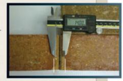
When the brick headers are separated by a standard mortar joint distance of 10 mm, the edge of the face of the brick could appear to be separated by a maximum of 25 mm when the corner texture is fully filled in. This will lead to the appearance of thick joints at the face, while the actual mortar joint is approximately 15 mm thinner.
